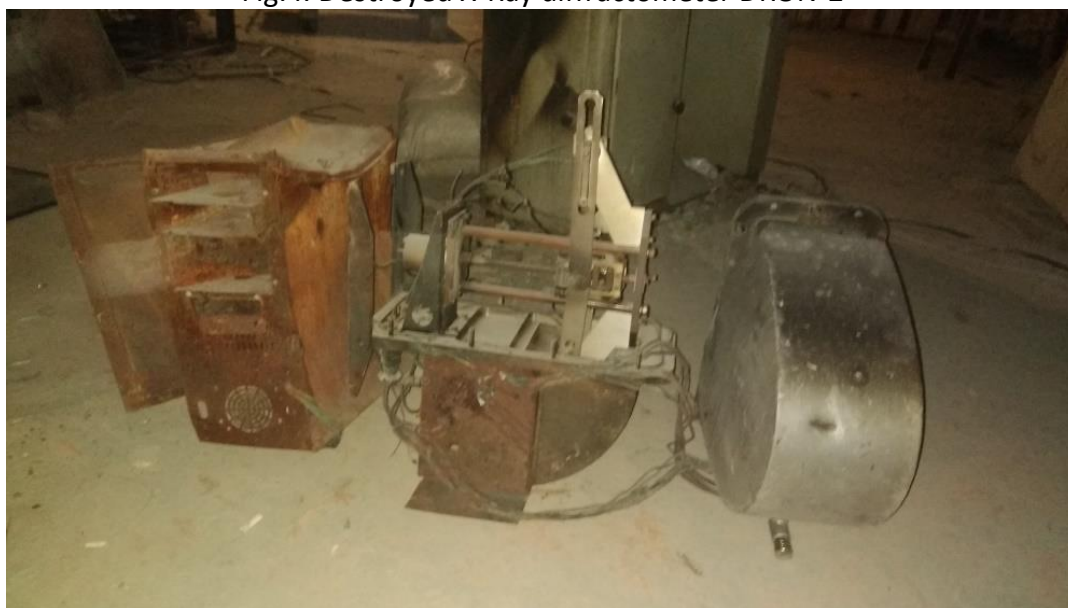
Fig.5. Burnt XRF spectrometer SPRUT-M
