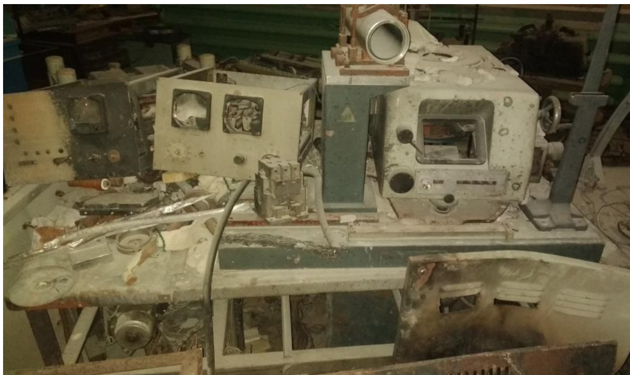
Fig.4. Destroyed X-Ray diffractometer DRON-2
